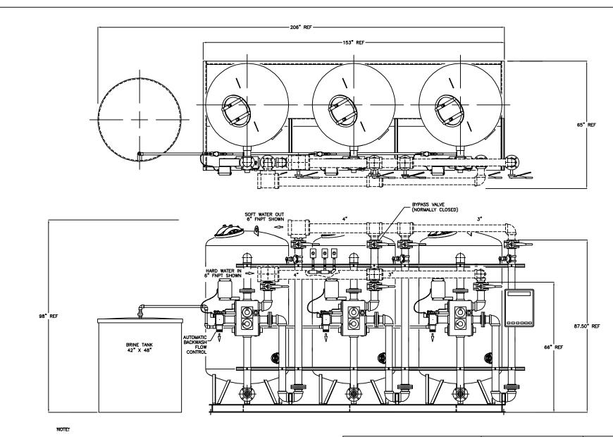
1. ALL PIPING, FITTINGS, VALVES, ETC. SHOWN IN BROKEN LINES ARE SUPPLIED BY OTHERS DIMENSIONS MAY CHANGE UPON FABRICATION. ALL DIMENSIONS ARE ±1"
